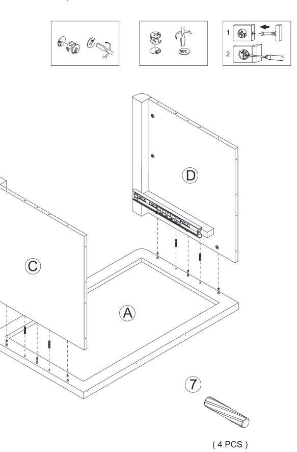
Insert four WOODEN DOWL (7) to the ENDS(C and D). Attach the BOTTOM (B) to ENDS (C and D) by using six PEN HEAD SCREW (8).
