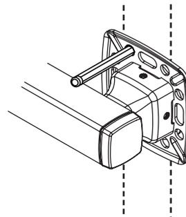
Place grab bar and mark three mounting locations on each of the two grab bar flanges with a pencil. (Refer to figure #2)
