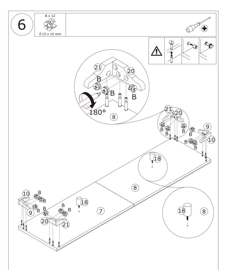
Attach panel 9, 10, 20 and 21 to panel 7 and 8, add cam lock(B) into panel 9, 10, 20 and 21 and turn clockwise to tighten as shown. Fix leg 18 to panel 7 and 8 as shown.
