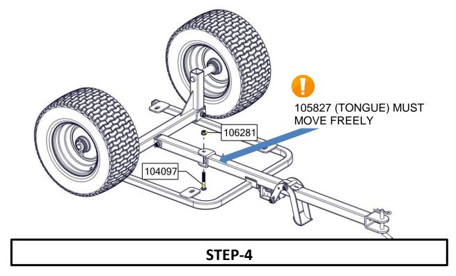
1. INSTALL BASE TO FRAME ASSEMBLY WITH ALL FASTENERS AS SHOWN AND **SECURELY TIGHTEN FASTENERS.**
