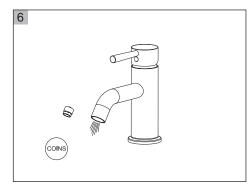
After installation is complete, remove aerator and rotate handle to the closed position. Turn on the water supply valves, and check all connections for a leak. Turn on your faucet and allow both hot and cold water to run at least one minute each. Replace Aerator.
