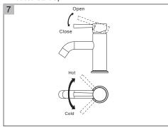
Lift the handle up, the cartridge will be activated allowing water to flow. The water flow will increase by continuing to rotate handle. By rotating the handle to the right, the water temperature will decrease to cold flow only. By rotating Handle to the left, the water temperature will increase to hot only.
