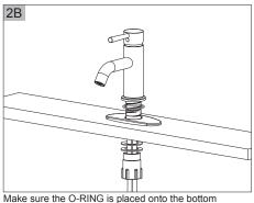
of Base Ring, Install faucet through Deck Plate. From underside sink, put Plastic Washer and Mounting Nut. Position faucet on sink properly and tighten Mounting Nut.
