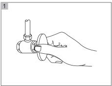
You should clean all the dirts from valve outlets. Turning off the water supply valves. This is usually found near the water meter. If you are replacing an existing faucet, remove the faucet from the
