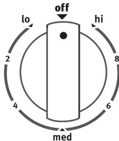
The control knobs can be set to anywhere between Hi and Lo. Push in and turn to setting.
