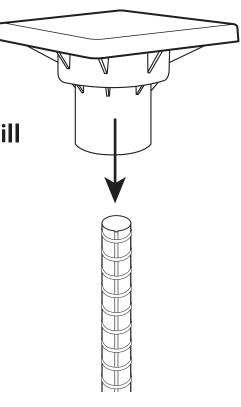
Push OSHA cap onto rebar Accepts #3 - #6 rods
