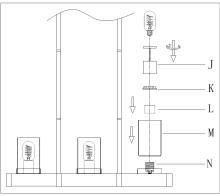
Unscrew the socket ring (K) and sleeve (L) from the socket(N). Gently and carefully position glass (M) and sleeve (L) onto the socket (N), then use the spacer (J) to thread the socket ring (K)till snug for securing the glass shade in place . Install the bulb (not included) (Please do not exceed the maximum
