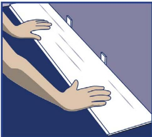
**Step 1: Begin installation working from left to right. Insert spacers at ends and edges where flooring meet wall.**
