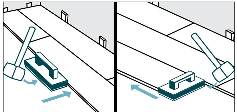
**SMART TIP** Use a scrap piece of plank to keep the joints lined up. This is called a "bridge."
