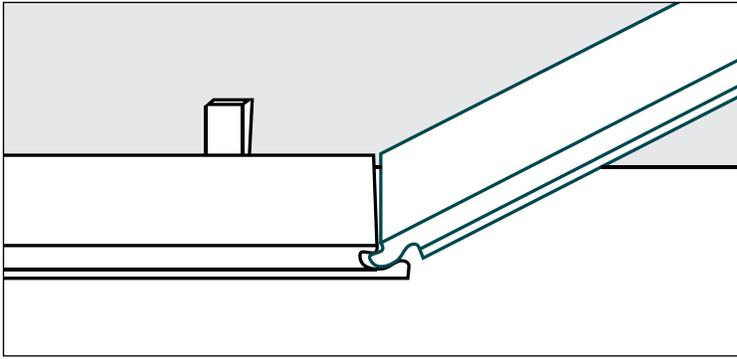
**STEP 8** Start your second row. With a cut-off that is more than 8" long or start with a new plank.
