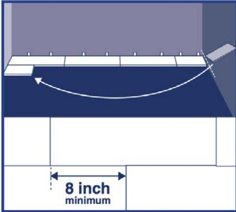
**Step 3:** Use leftover flooring from first row as starter for second row. There must be at least 20cm between flooring end joints on adjacent rows. **FOR TILE INSTALLATIONS:** The distance between end joints should be
