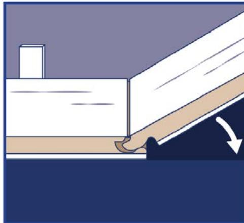
**Step 2: Lock short end of flooring by inserting tongue into groove at an angle and drop in place. Continue to end of first row.**
