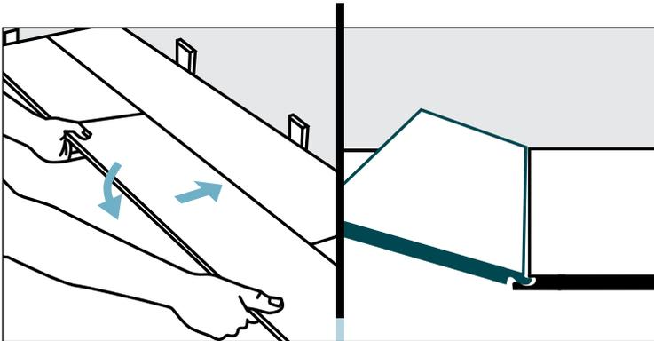
**STEP 10** Tap the length end to ensure a tight fit, then tap the short end to drive down the short end tongue into groove.
