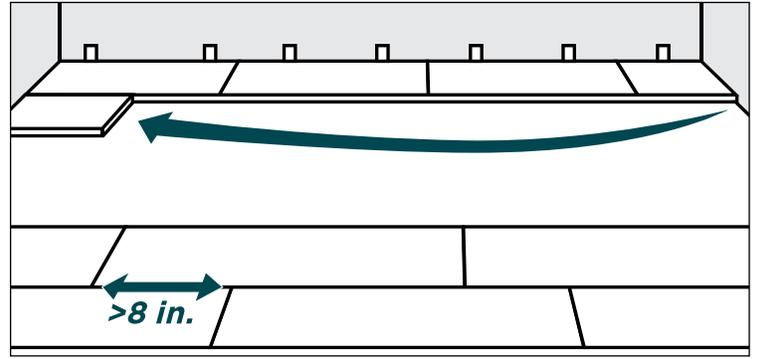
**SMART TIP** Remember to stagger end joints from row to row - 8+" for planks and 12+" for tiles.
