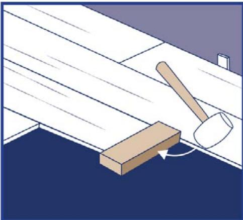
**Step 7:** Tap end of flooring with hammer and tapping block to lock ends of flooring together. Remove bridge and continue towards wall until installing the final flooring in the row. **BE SURE TO TAP ON EDGE OF**
