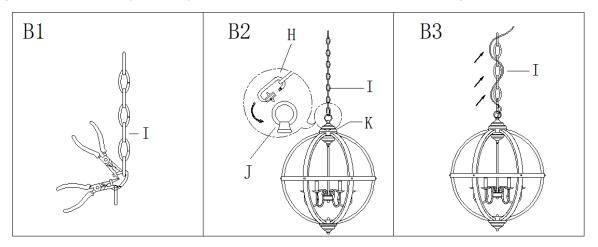
Step B1: By measuring, determine the correct number of links needed for proper hanging height. Using the chain pliers, disconnect and discard the remaining chain.
