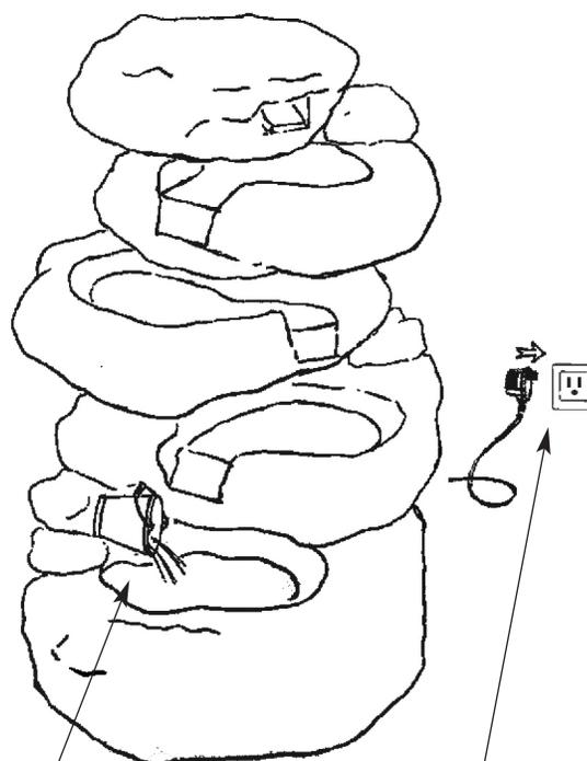
Adjust the pump flow rate to achieve the desired effect and to minimize any splashing. Splashing can occur if the flow rate is too high or the feature water level is too full. The flow rate can be increased or decreased by moving the flow rate control slider on the pump body. Moving the switch towards (+) will increase the flow rate and moving it towards (-) will decrease it.
