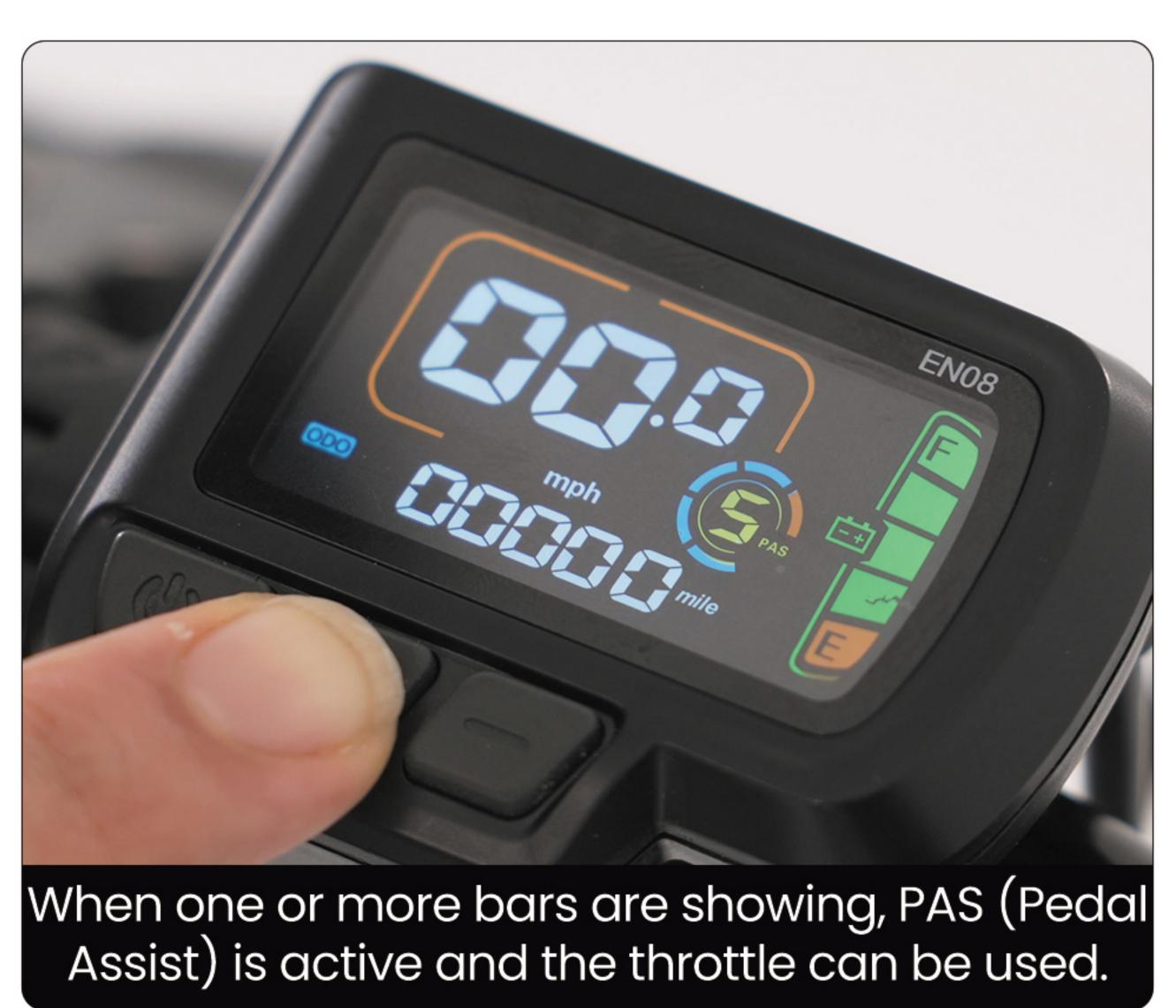
When you turn on the display, the PAS level is automatically set at 0, meaning no Pedal Assist (PAS) and no power to the throttle.
