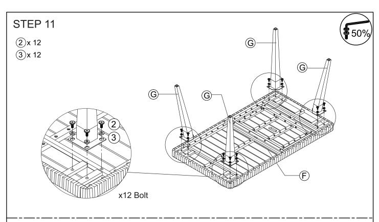
Connect the top table (F) & leg table (G), tighten bolt (2), flat washer (3) with allen key (5).
