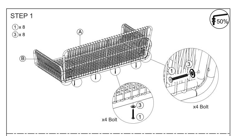
Connect the back (A) & seat (B), tighten bolt (1), flat washer (3) with allen key (5).
