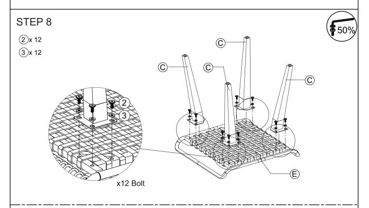
Connect the seat stool (E) & leg (C), tighten bolt (2), flat washer (3) with allen key (5).
