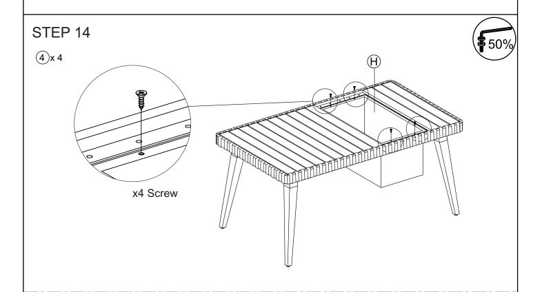
Connect the part from STEP 13 & box (H) with screw (4)
