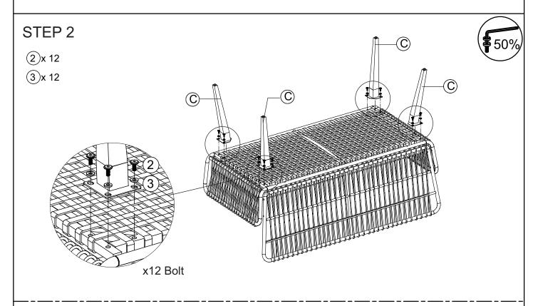
Connect the part from STEP 1 & leg (C), tighten bolt (2), flat washer (3) with allen key (5).
