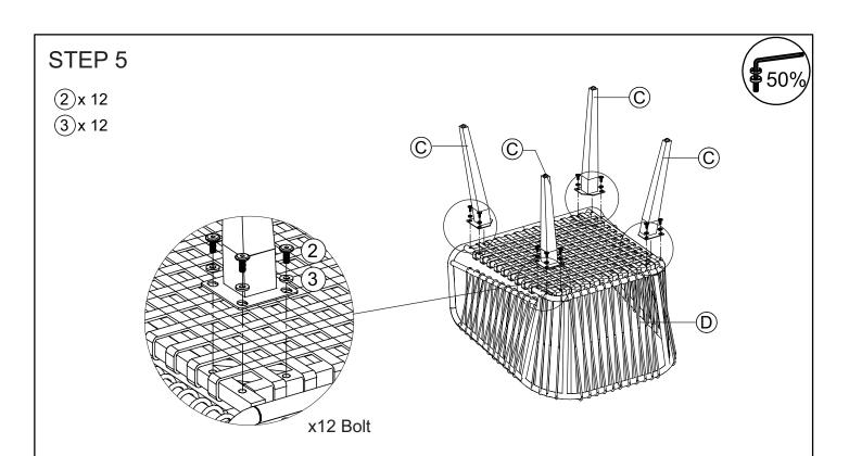
Connect the chair (D) & leg (C), tighten bolt (2), flat washer (3) with allen key (5).
