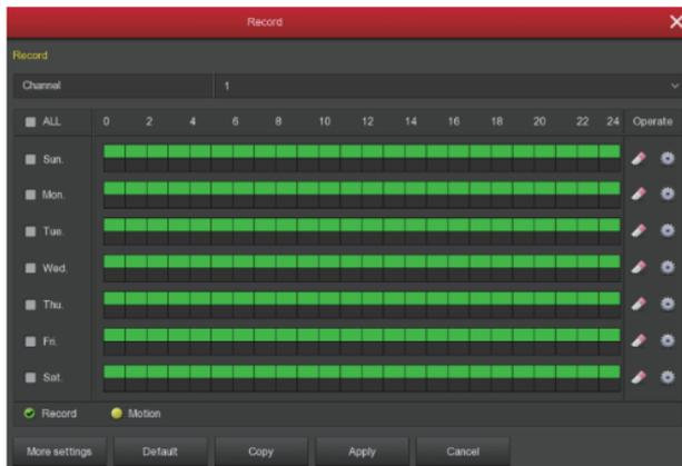
3、Motion Detection Setting. Enable "Motion" to activate motion recording, motion sections have no more than 6 times each day. If the setting of manual record and motion record are overlapped, it can only save the motion records while motion detection comes up.
