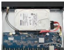
(3) Connect one end of the hard disk power cable and SATA data cable to the motherboard and the other end to the hard disk.
