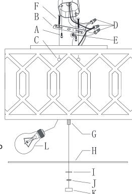
PLEASE USE TYPE"A" BULB MAX 60-WATT OR CFL BULB MAX 13-WATT OR LED BULB MAX 9 -WATT THERE ARE 2PCS 9-WATT LED BULB IN THE BOX
