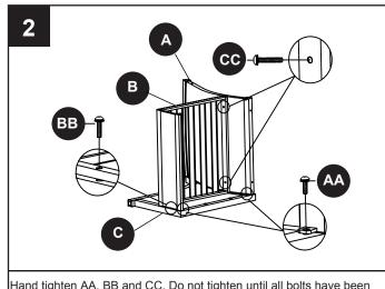
Hand tighten AA, BB and CC. Do not tighten until all bolts have been installed
