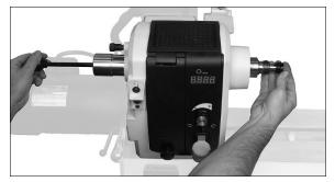
Figure 7-8: removing spur center
