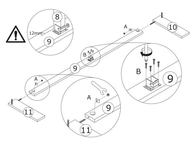
Attach plate 10 and 11 to plate 9 using part(A) as shown. Fix iron part(B) to plate 9 as shown.
