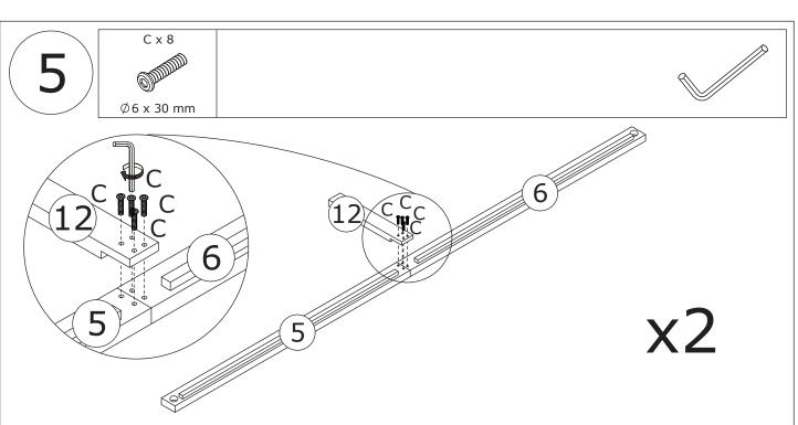
Fix plate 12 to plate 5 and 6 using screw(C) as shown.
