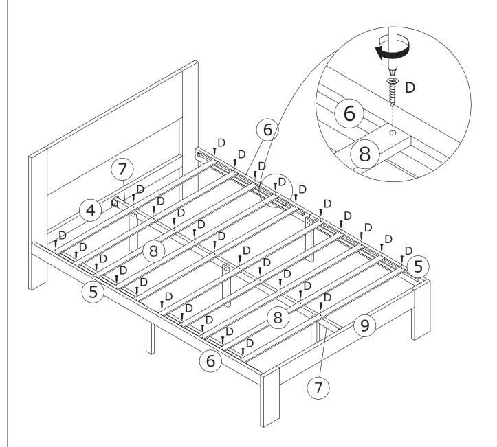
Fix plate 8 to the component using screw(D) as shown.
