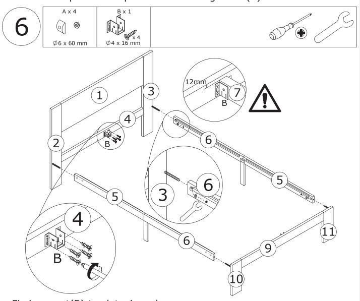
Fix iron part(B) to plate 4 as shown. Connect plate 5 and 6 to plate 2, 3 and 10, 11 using part(A) as shown.
