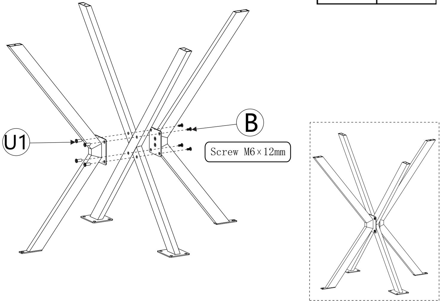
EN-During the assembly, please first half-tighten all the screws into the holes.
