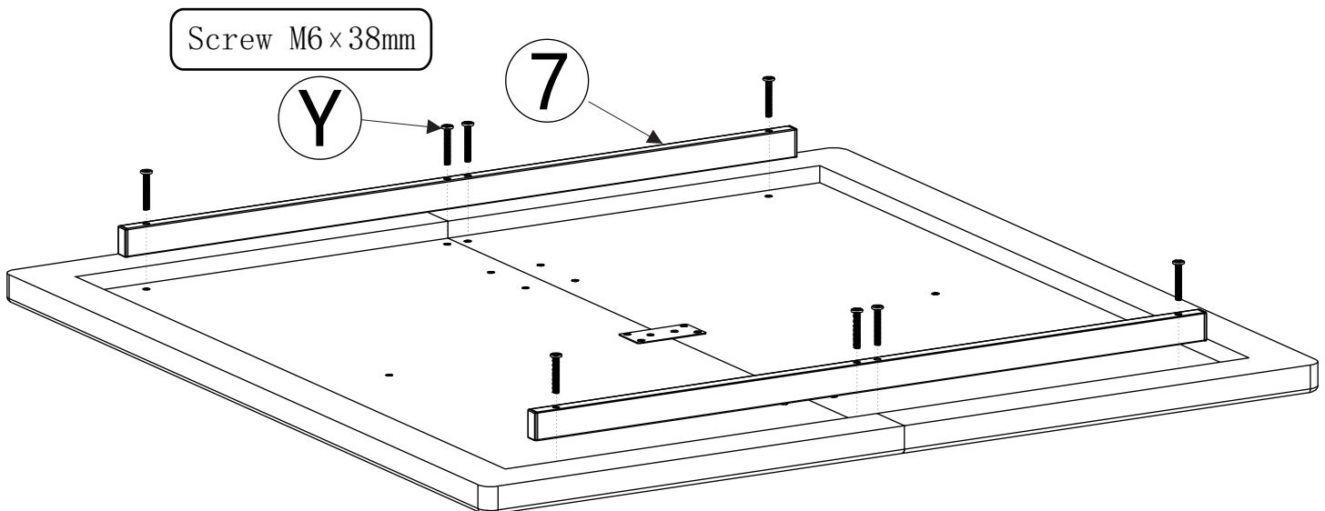
EN-During the assembly, please first half-tighten all the screws into the holes.
