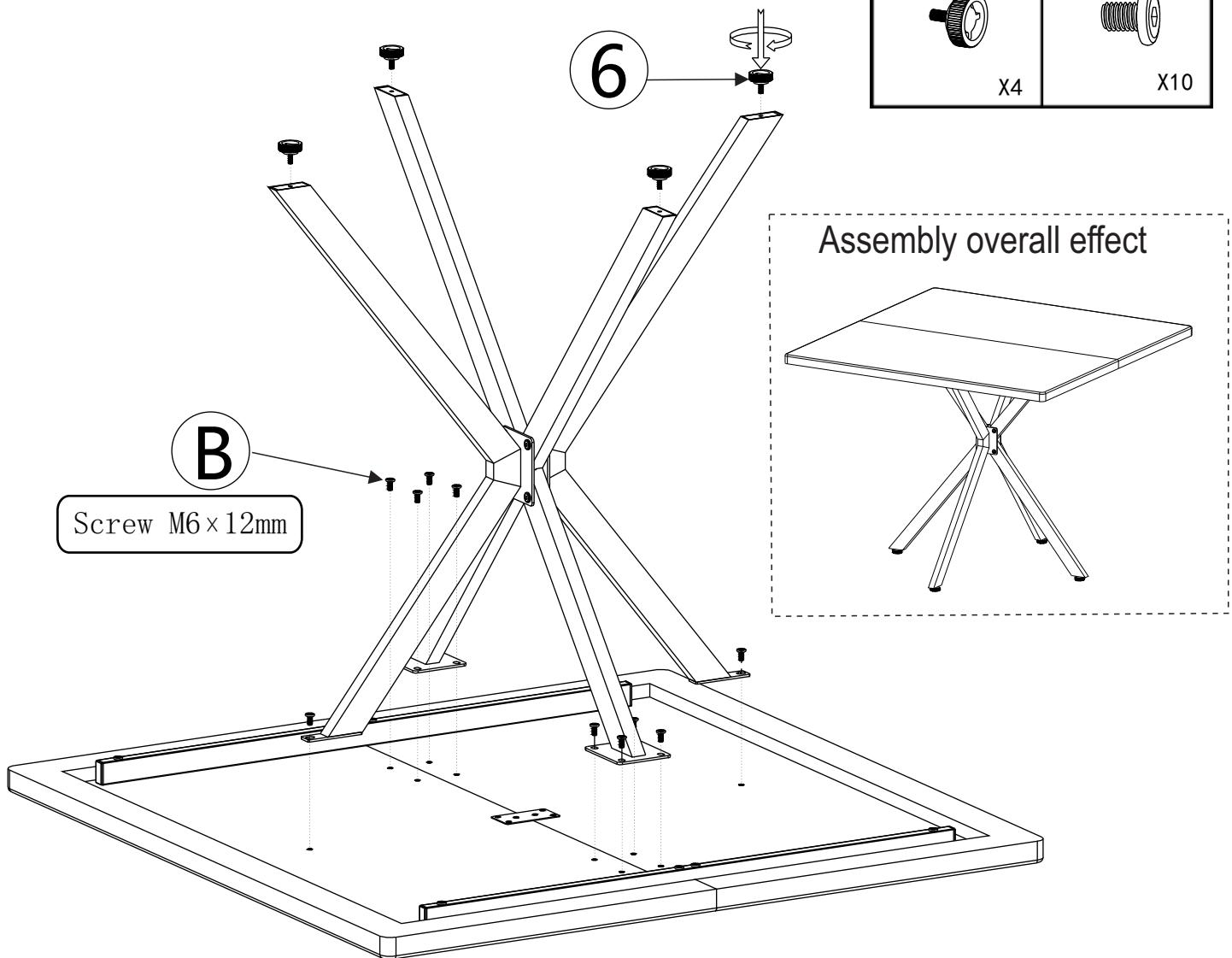
EN-During the assembly, please first half-tighten all the screws into the holes.
