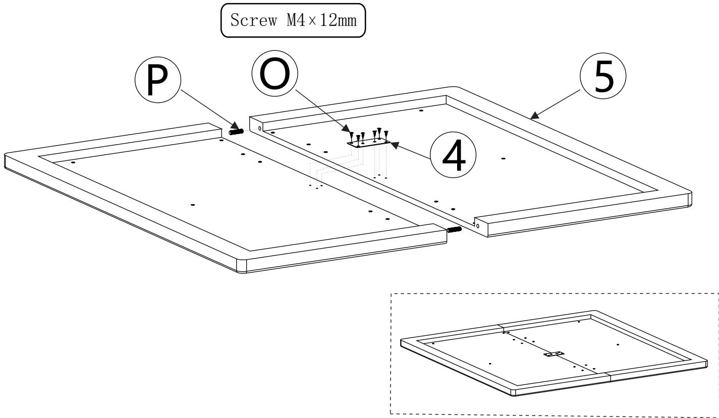
EN-During the assembly, please first half-tighten all the screws into the holes.
