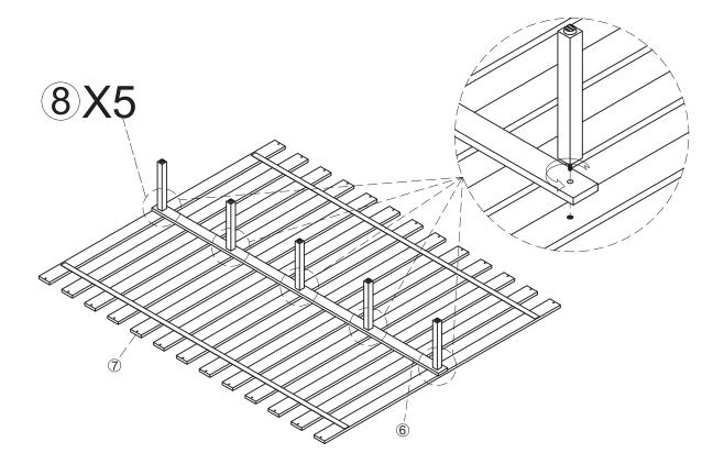
Adjust the leveling feet of the legs ® to ensure all slats ⑦ are leveled and staying at the same level.
