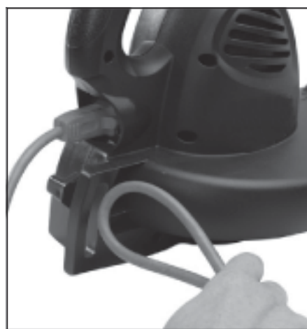
Figure 4 - Inserting extension cord loop through cord slot
