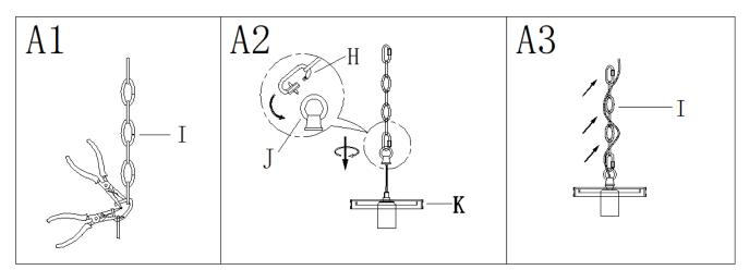
Step A1: By measuring, determine the correct number of links needed for proper hanging height. Using the chain
