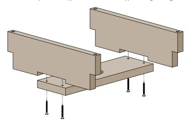
**Note:** The bottom support board should \*NOT\* sit flush with bottom of the side supports:
