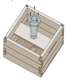
13. Slide your light pole, umbrella, or other pole into the metal tube and secure by tightening the wingnut. To stabilize the planter, we recommend adding gravel until it reaches the top of the support beam and then add potting soil above. This will allow for the best drainage while still giving you the ability to grow beautiful plants.
