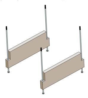
4. Slide the assembly created in steps 1 and 2 on top of the bolts and all the way down.
