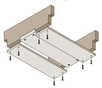
**Note:** There should be a small gap between the boards – this is normal and is designed to help with drainage.
