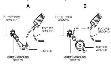
Connect wires according to the below chart
