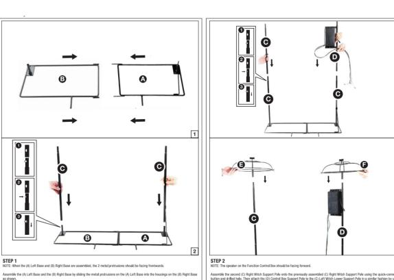
Then assemble one of the (C) Right Witch Support Poles to the (B) Right Base using the quick-connect push button and drilled hole. Assen the (C) Left Witch Lewer Support Pole to the (A) Left Base in a similar fashion by using the quick-connect push button and drilled hole as sh
