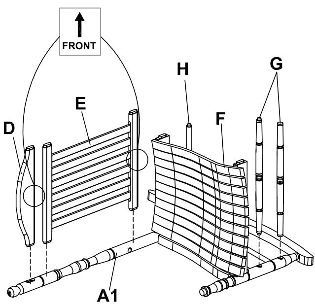
Attach the top back support (D), back support (E), seat (F), front cross bar (G), and back cross bar (H) into right side frame (A1).
