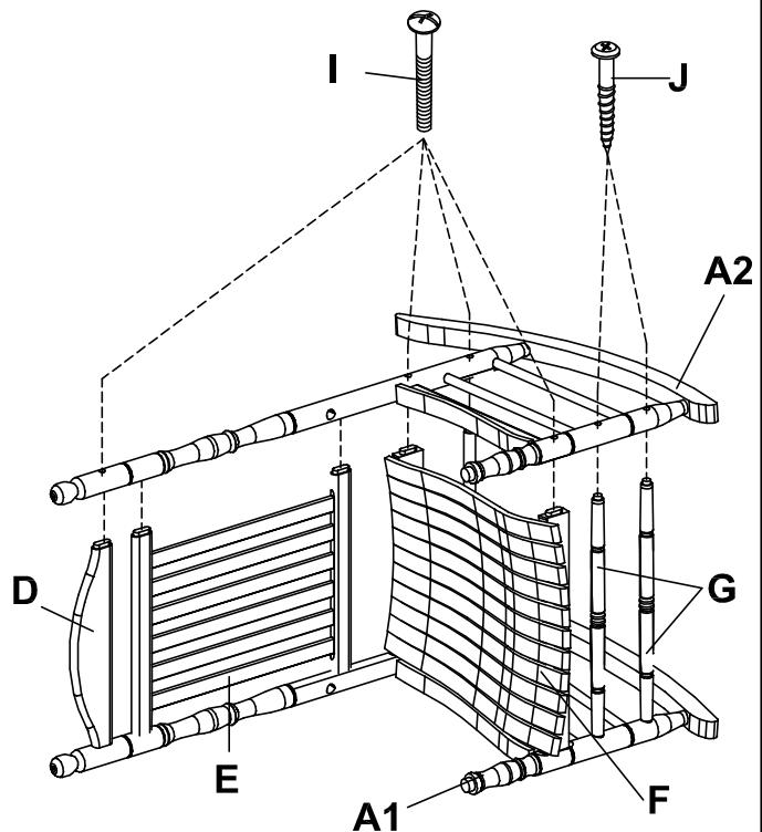
Attach the left side frame (A2) into assembly. Insert bolts and screw into predrilled holes, and tighten to secure using 1 1/2" bolt (I) and 1 3/4" screw (J).
