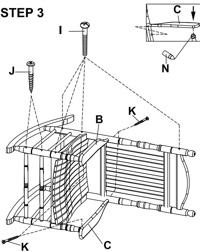
Pour small of glue (N) into arms hole (B & C). Attach arm rest (B & C) to right side frame (A1) and left side frame (A2). Secure using 1 1/2" bolt (I) 1 3/4" screw (J) to right side frame (A1). Next, secure using 1 1/2" screw (K) to right and left side frame (A1 & A2). Tighten all screws and bolts using screwdriver.
