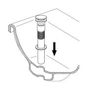
2. Put the pop up drain stopper into sink hole
