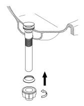
3. Re-screw the bottom washer and lock nut onto drain stopper
