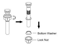
1. Unscrew the lock nut and bottom washer from drain stopper
