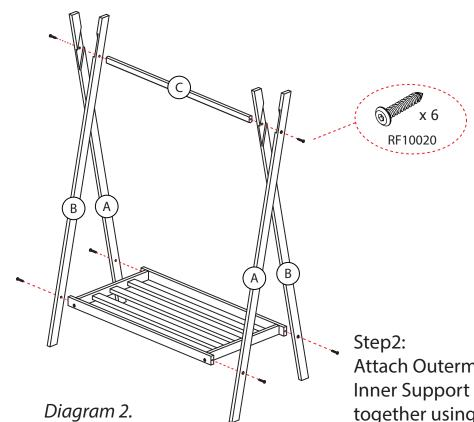
Attach Outermost Support Beam (A), Inner Support Beam (B) and Wood Bar (C) together using screws (RF10020) as per diagram 2.
