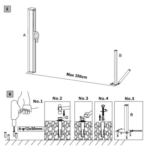
Installed on the concrete floor as shown in the figure above.
