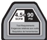
**IMPORTANT:** To operate correctly, this tool requires airflow that is at least 4.5 Standard Cubic Feet per Minute (SCFM) at 90 pounds per square inch (PSI). Check the specifications of your air compressor to be sure that it can support both the minimum SCFM and PSI required. The air hose length could affect how much air pressure the tool is actually receiving. You may need to adjust the air pressure higher on the air regulator to achieve the working pressure of 90 PSI.
