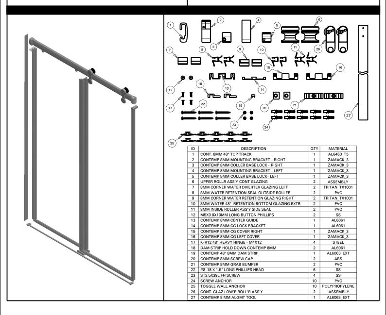
MATERIALS: Anodized Aluminum Extrusions (Track) and Zinc Die Cast (Mounting Brackets).
