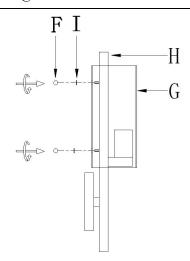
4. Attach the mounting plate assembly (A) to outlet box with mounting screws (C). Carefully pass the supply wires through the mounting plate assembly (A).
