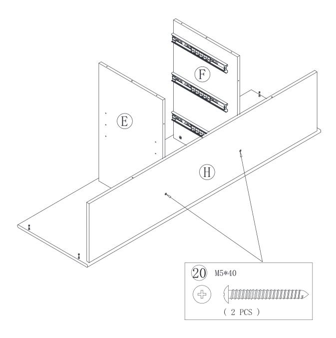
Insert three WOOD DOWELS (10) to the UPPER BACK (H). Attached the LOWER BACK to the UPPER BACK (H).
