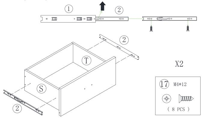
• Fasten two EXTENSION SLIDES (2) to the DRAWER SIDES (S and Z). Use four FLAT HEAD SCREWS (17) through the exact holes shown.
