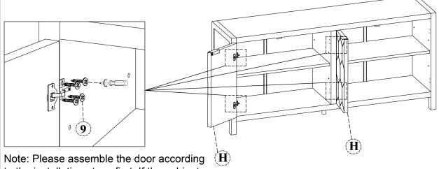
Note: Please assemble the door according to the installation steps first. If the cabinet door is deviated, the internal hinge needs to be slowly adjusted to solve the problem.
