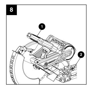
**CAUTION:** To avoid injury and damage to the saw, transport and store the miter saw with the cutting head locked in the down position. Never use the stop latch to hold the cutting head in a down position for cutting operations.
