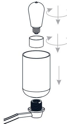
Install four correct bulbs referring to fixture markings and/or labels for maximum wattage.
