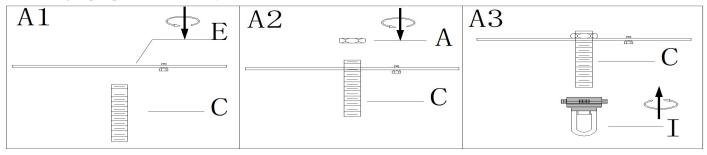
Step A1: Thread the single bar(E) onto nipple (C),
