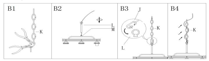
Step B1: By measuring, determine the correct number of links needed for proper hanging height. Using the chain pliers, disconnect and discard the remaining chain.
