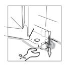
When the refrigerator stays in the packing box, plastic feet are in tightened state. After carrying it out from the packing box for placement, please make sure to adjust two front plastic feet until the height is suitable; just adjust two plastic feet with a wrench or directly by hand.
