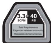
**IMPORTANT:** To operate correctly, this tool requires airflow of at least 3.3 cubic feet per minute (SCFM) at 40 pounds per square inch (PSI) at the tool. Check the specifications of your air compressor to be sure that it can support both the minimum SCFM and PSI required. The air hose length could affect how much air pressure the tool is actually receiving. You may need to adjust the air pressure higher on the air regulator to achieve the max working pressure of 40 PSI.
