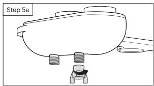
**IMPORTANT:** Failure to connect or cap the hot water supply will result in leaking during use.
