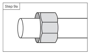
b. Push the hot water flex tubing over the pressure connector.
