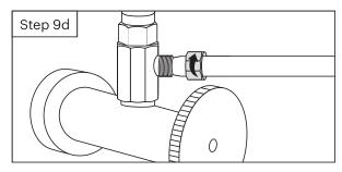
**CAUTION:** Do not overtighten the pressure cap. You will risk damaging the tubing.
