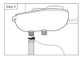
**NOTE:** If you have already installed the hot water supply cap over the hot water supply on your SSE-25 Dual Temperature model, skip to Step 5 on Page 11. Otherwise, proceed to the next steps.
