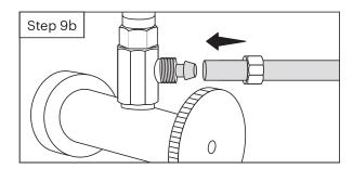
**IMPORTANT:** Be sure to slide the hot water flex tubing over the pressure connector until the tubing slides past the "lip" of the pressure connector and it cannot go any further.
