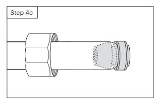
**NOTE:** If there is any leaking, check all rubber washers and make sure all water connections are tight and secure. If necessary, wrap Teflon tape around the threading of any leaking connections.
