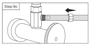
d. Screw the cap onto the T-Valve until secure and tight.
