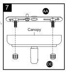
NOTE:Depth of threaded pipe may need to be adjusted to properly fit fixture, decorative cup and finial.
