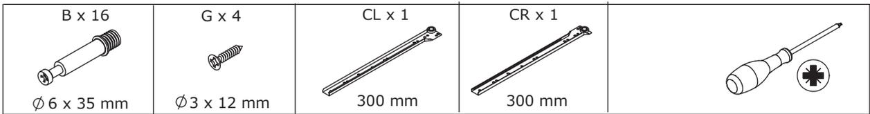
Screw eccentric rod(B) into board 8, and fix rail(CL) and (CR) with screw(G) at first.
