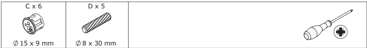
Attach board 2, 13 and 14 to board 9 using wooden dowel(D), add cam lock(C) into and turn clockwise to tighten as shown.
