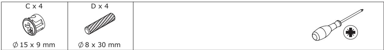
Attach board 1 to board 6 and 7 using wooden dowel(D), add cam lock(C) into and turn clockwise to tighten as shown.
