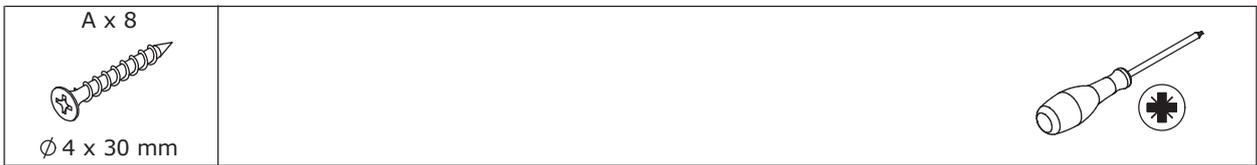
Fix board 17 and 18 to board 23 with screw(A) as shown.
