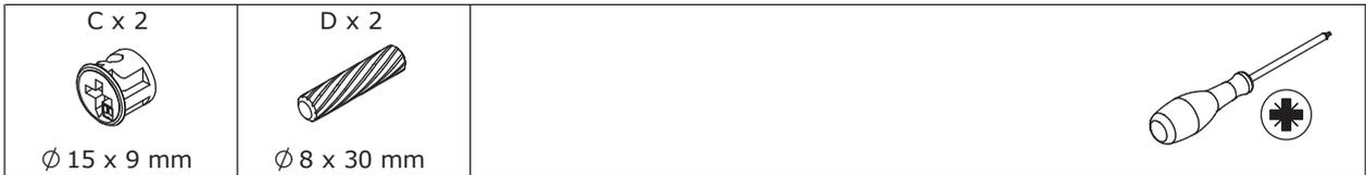
Attach board 3 to board 10 using wooden dowel(D), add cam lock(C) into board 10 and turn clockwise to tighten as shown.
