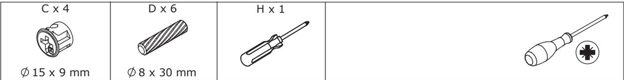
Attach board 5 to board 16 and 4 using wooden dowel(D), add cam lock(C) into board 4, 16 and turn clockwise to tighten as shown.
