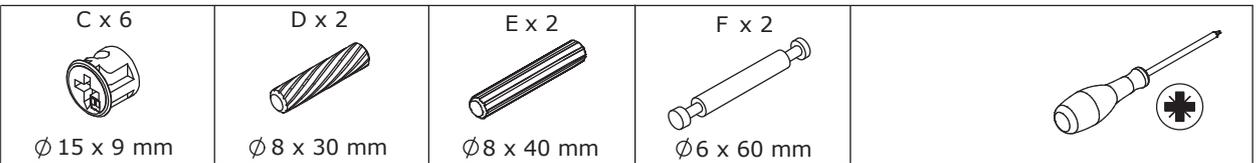
Attach board 3 to board 4 using wooden dowel(D), add cam lock(C) into board 3 and turn clockwise to tighten at first.
