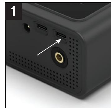
**IMPORTANT: Use a 5V3A adaptor for fastest charging. Using 5V2A will take longer to charge.**
