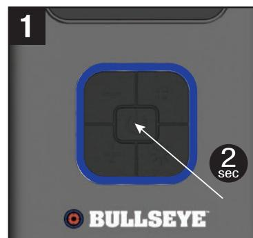
On the Control Panel, **press and hold down the
