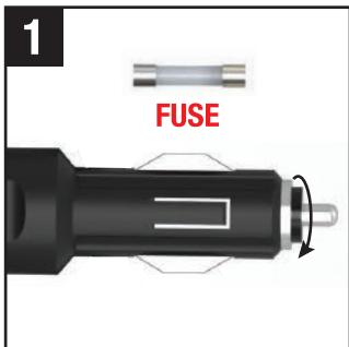
Carefully unscrew the front washer from the 12V DC Car Power Cord (it is spring loaded).
