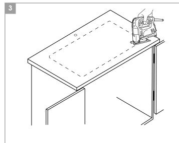
Trace the outline of the template and cut countertop according to templated outline using appropriate cutting tools. Template is for guide only. Use physical sink to ensure accurate cut-out opening.
