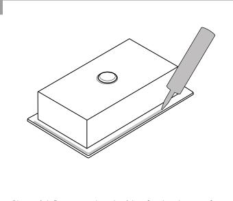
Clean sink flange and underside of cut-out area of countertop, making sure that the area is smooth and free of debris. Apply continuous bead of silicone.
