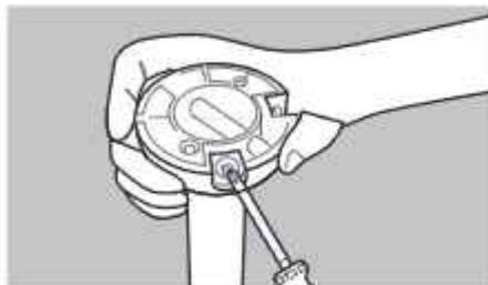
❶ Loosen the screws on the hanging ball.
