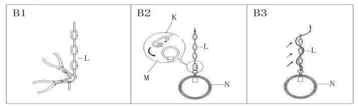
Step B1: By measuring, determine the correct number of links needed for proper hanging height. Using the chain pliers, disconnect and discard the remaining chain.
