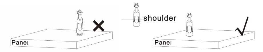
Tighten quickfit until shoulder is flush with panel. Do not overtighten or undertighten.
