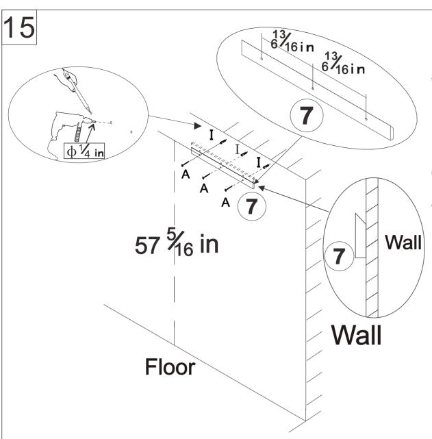
Install the hanging rail (#7) onto the wall first. There are 3 Pre-drilled holes provided on the Hanging Rail for drilling directly into the wall. If the location of these pre-drilled holes do not line up with your studs, please drill new holes into the hanging rail, to line up with the location of your studs.
