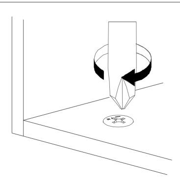
Turn cam lock clockwise to tighten.
