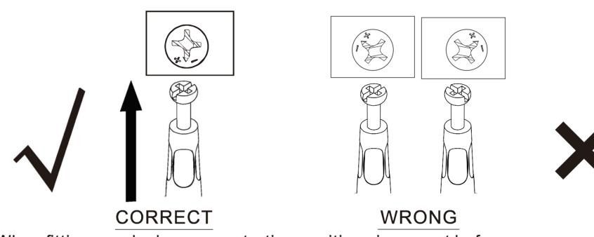
When fitting cam lock, ensure starting positions is correct before you insert cam lock to quickfit.
