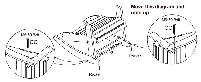
NOTE: Bolt only goes from the outside through the Rocker into the Crossbeam.
