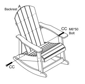
Attach the rear of the Left Armrest (Part C) and Right Armrest (Part D) to the Rear Legs (Part F) and Backrest (Part A) using (2) M6\*70 Bolts (Part EE).
