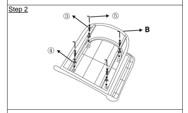
Attach Base(B) and Seat(A) using Bolts( $\mathfrak{I}$ ) and Washers( $\mathfrak{I}$ ) with Allen Key( $\mathfrak{I}$ ).
