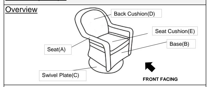
This Swivel Chair has multiple parts and may require up to 30 minutes to assemble. To give you an overview of the Swivel Chair parts, the above picture is to help you put the various parts into perspective. Please read through the instructions below to familiarise yourself with the parts and steps before assembly.
