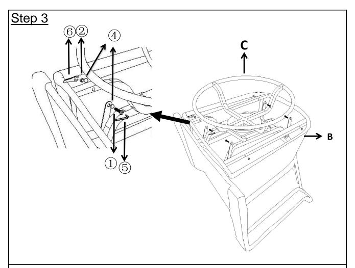
With the help of and adult partner, place the Chair Body facedown. Attach Swivel Plate(C) to Base(B) using Bolts( $\widehat{1}$ ), Washers( $\widehat{4}$ ) and Nuts( $\widehat{2}$ ) with Allen Key( $\widehat{5}$ ) and Wrench( $\widehat{6}$ ).
