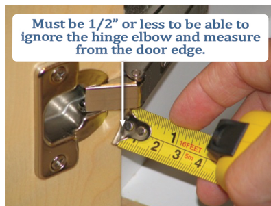
You can take advantage of the space created under the protruding hinges as long as the elbow doesn't protrude into the opening more than 1/2 inch.
